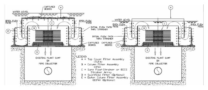
Upon recirculation start up; and for some period of time, most of the fluid flow is through the filter panels to the strainer(s). As the filter panels trap debris, the volume of flow through the open flow path will increase. As long as the fluid flow continues through the filter panels at some level, the panels will continue to remove and trap fibrous debris including fines suspended in the water column.
