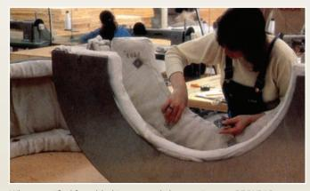
When specified for added impact and abuse resistance, RE/WRAP insulation components can be supplied with metal jackets having quick release latches to make removal and reinstallation fast and easy. In the case of this component, RE/WRAP insulation blankets have been permanently affixed within the metal jacket; a single operation takes care of removal or reinstallation of both jacket and insulation as one unit.
