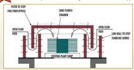
Sure-Trap™ is a series of filter panels positioned around a strainer that will trap fibrous debris, specifically <u>FINE</u>
